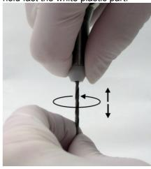
Apply only slight pressure when inserting the drill. The stuck dust will come loose and by turning the drill it will come out. During this procedure hold the handpiece upside down so that the dust can fall down easily. After that screw on the metal sleeve again.
