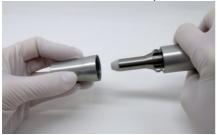
Clean the inside of protective sleeve and the hull with a dry scrubber or brush. Now insert carefully the provided special drill into the handpiece.
