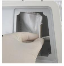
The micro filter (art. 5179) must be used. The control unit filter (art. 5115) must
