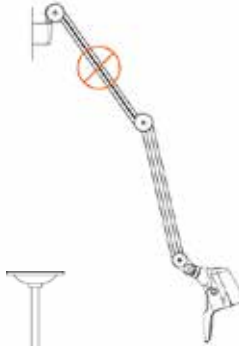
Arm under lower work area. Overload of arm.
