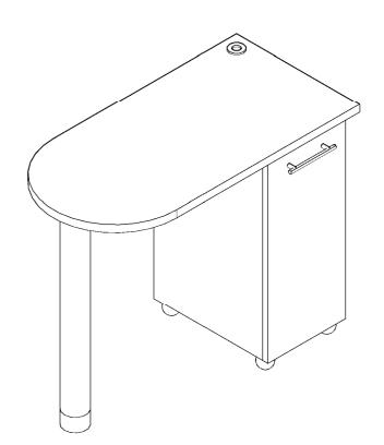
2. If the unit feels uneven, this can be corrected by turning the adjustable foot on the Leg (B).
